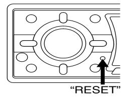
The RESET button is located in front of the panel. It is recessed in order to prevent accidental engagement, and can be activated with the tip of a ball-point pen or any similar pointed object. This reset circuitry is provided in order to protect the unit's microprocessor, and should only be activated under the following conditions:
